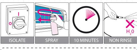
Isolate electrics. Spray into coil, starting at top corner and methodically working across and down. Keep all surfaces wet for 10 minutes. Ensure EasyCare™ penetrates completely through coil. No rinsing required.
